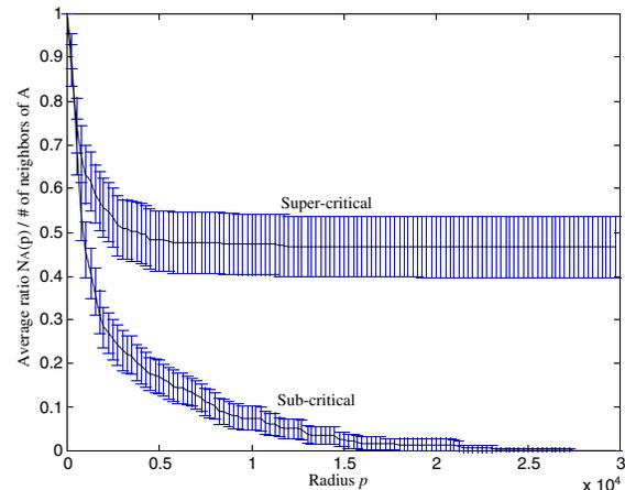
Fig. 3. Average ratio between  $N_A(p)$  and the number of neighbors of  $A$  for sub- and super-critical densities. For sub-critical densities,  $N_A(p)$  goes to zero, because  $A$  belongs a.s. to a bounded cluster. For supercritical densities,  $N_A(p)$  tends to a limit  $N_A^\infty$  noticeably smaller than  $\lim_{p \rightarrow 0} N_A(p)$ .
